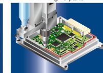
Liquid gasket sealing of an ECU
