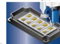
Dispensing solder paste on IGBT modules
