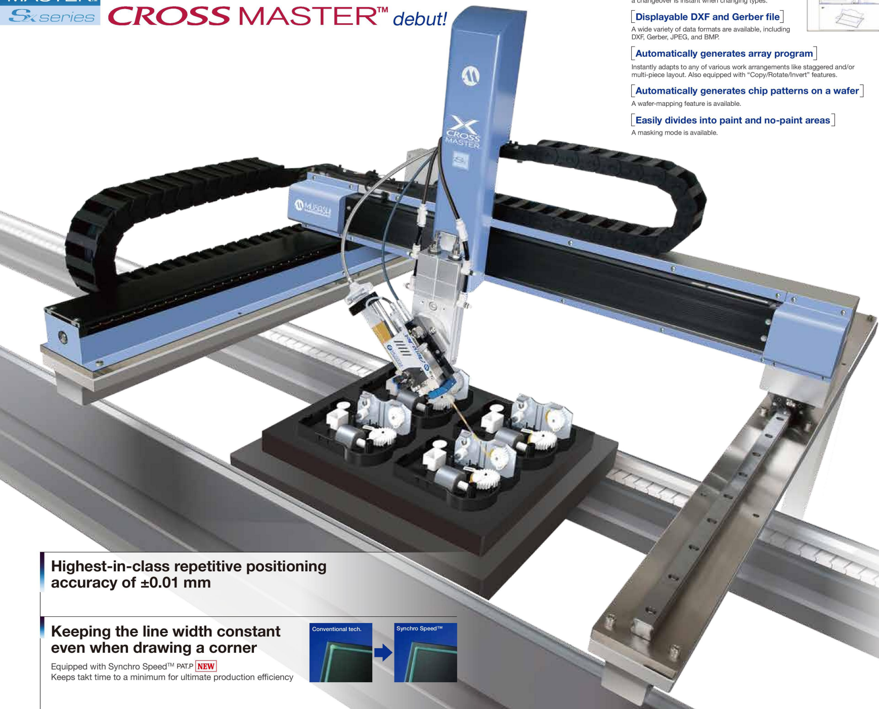
Dispensing solder paste on IGBT modules
