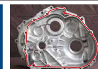
Liquid gasket sealing of an engine parts
